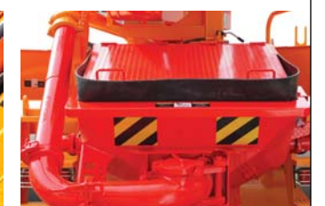
▲large capacity hopper
