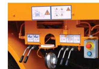
▲control v/v for outrigger
